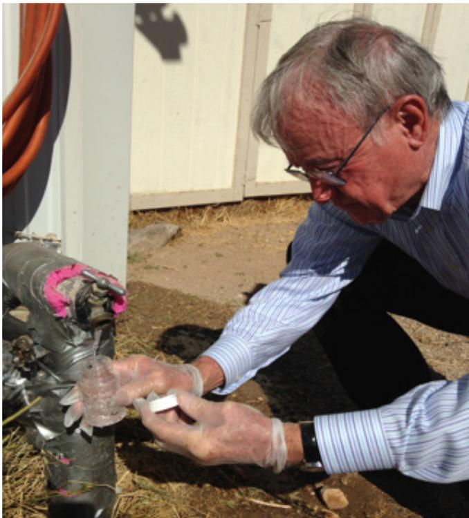
Figure 3. Author demonstrating proper well water sample collection.
